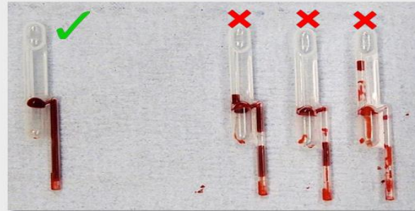
Pipette filled correctly
