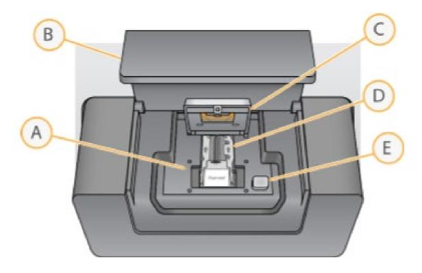
The flow cell compartment contains the flow cell stage, thermal station, and fluidics connections to the flow cell. The flow cell stage holds the flow cell and the flow cell clamp secures and positions the flow cell. When the flow cell clamp closes, two pins near the clamp hinge auto-position the flow cell. The thermal station, located beneath the flow cell stage, controls changes in flow cell temperature required for cluster generation and sequencing.
