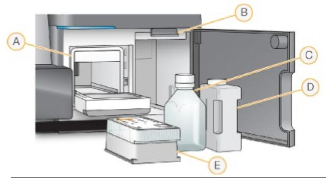
The reagent compartment contains the reagent chiller, and positions for the wash buffer (PR2) bottle and the waste bottle. To maintain a consistent temperature, open and close the reagent chiller only when instructed.
