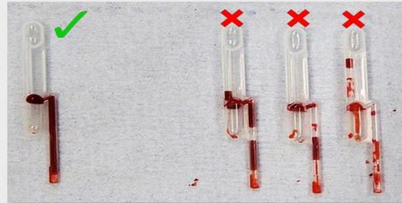
Pipette filled correctly
